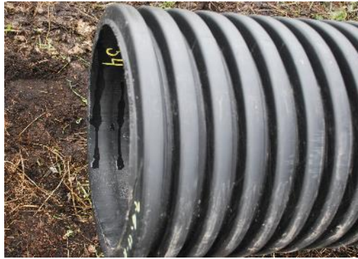
Figure 7: Double wall pipe
